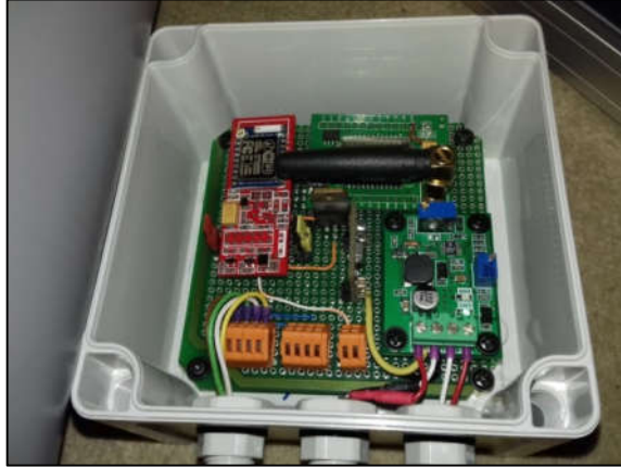
Fig. 6.6 Gateway circuits, in the enclosure.
