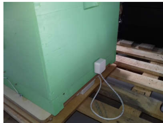
Fig. 7.8 Temperature sensor, between the hive bottom and the box.
