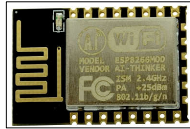
Fig. 3.63 ESP8266-12E module with PCB antenna and 4MB flash [13].
