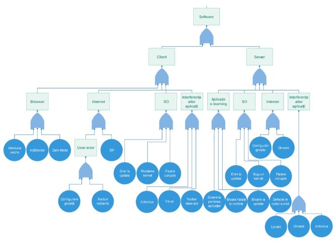
Fig. 3.13 Software Fault Sub-tree
