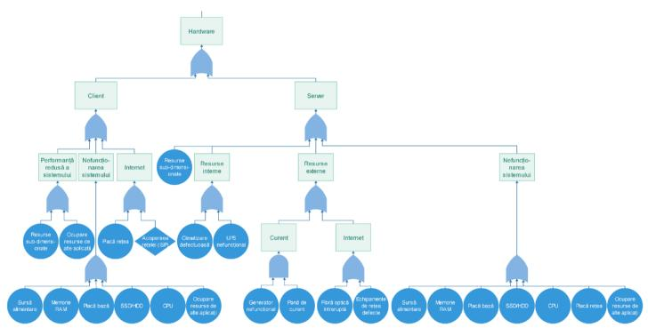
Fig. 3.14 Hardware Fault Sub-tree
